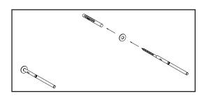
6. Next, put the washer onto the screw-end of the shelf brackets, and then insert the supports in to the holes, using a spanner to tighten them up sufficiently.
