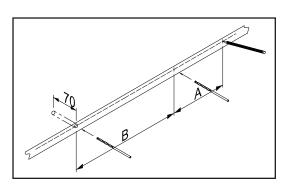
4. Insert your 10mm masonry drill bit in to the drill and make sure it is held in tightly. Be sure to use eye-protection, then drill a hole of 70mm deep at each point marked. Ensure the drill is straight and that you apply pressure evenly when drilling.
