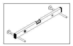
7. Use a spirit level to ensure that the brackets are pointing out of the wall straight and horizontally, so that you can be sure your shelf will sit flat.
