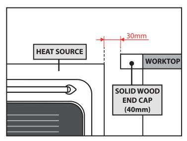
When a worktop is to be fitted near a freestanding oven (i.e. an oven that is not housed in a cabinet, such as a range cooker) allow a minimum gap of 30mm all the way around the worktop, and fit a solid wood end cap along the worktop edge. This will protect the end grain and help to prevent splitting.
