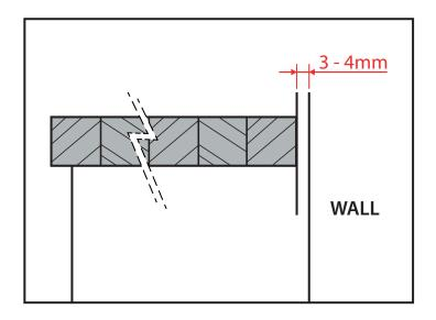
When positioning the worktop you must allow a 3-4mm gap between all worktop edges and any adjacent walls or units (particularly between the back of the worktop and the wall). This will allow the worktop to expand and contract with the humidity of the kitchen without causing damage.
