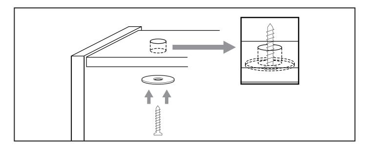
**IMPORTANT:** Do not screw through the carcass directly into the worktop. Do not use fixing blocks to secure. Do not use any worktop fixing methods other than those recommended here.
