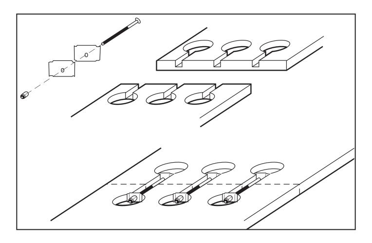
As a rule only Butt joints should be used on wooden worktops. However, if your worktop has a radius and you do have to use a mitre joint, ensure that the "hockey stick" does not over extend the 10mm bull-nose radius.
